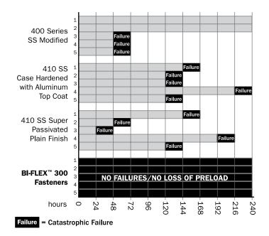
All fasteners were placed through a clear hole in 6061 T6 aluminum with a thickness of 0.125" and drilled into an unplated steel strip measuring a thickness of 0.125". A strip of 0.060" aluminum was placed in between the 0.125" aluminum and steel strip on one side, to simulate a fastener placed under load.
